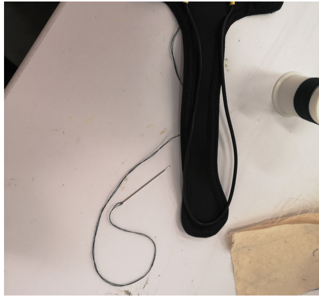
Hand sew loose lines to keep the rubber in place.
