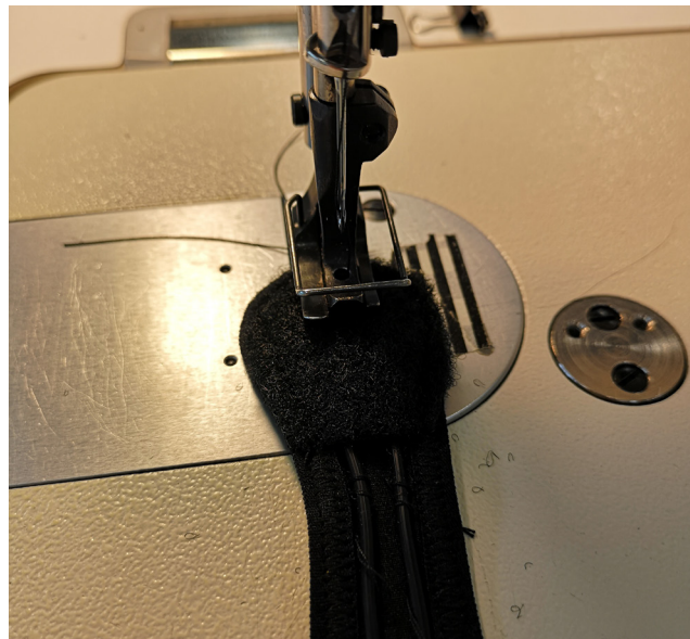
Sew lines at the middle to prevent rubbers touching each other.
