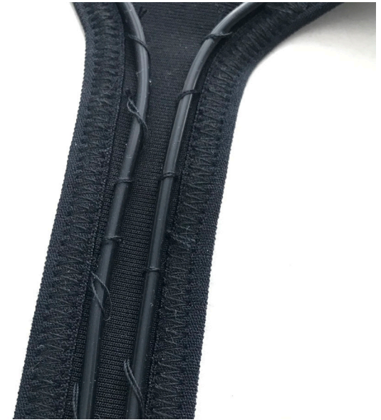
The loose lines prevent the rubber from touching together but save the elascity.
